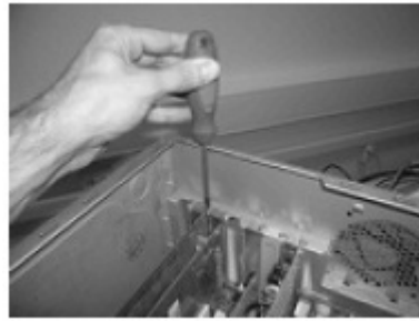
Example of FS-6C video capture card installation into a PCI slot.
