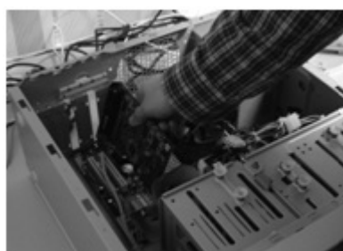
Example of FS-16 video capture card installation into a PCI-E X1 slot.
