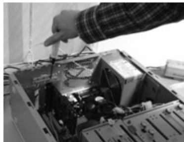
Example of FS-16 video capture card installation into a PCI-E X1 slot.
