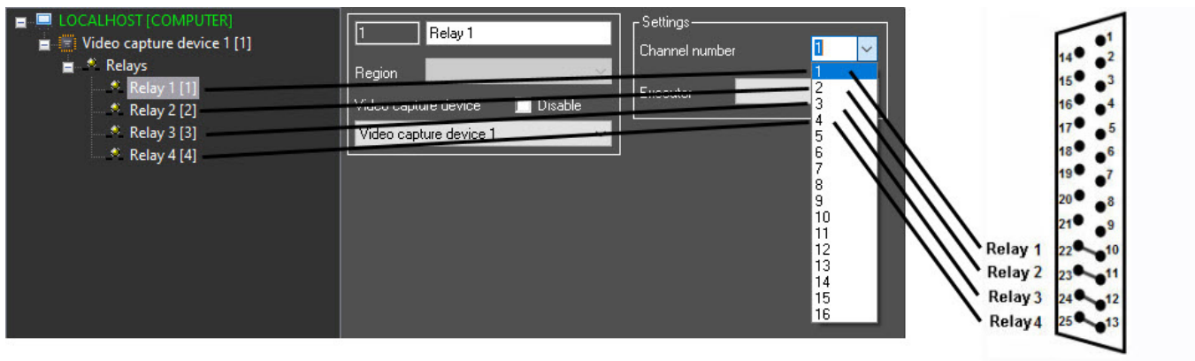
Channels of the second 4/4 Sensor-Relay card (low profile) are numbered 1-4.
