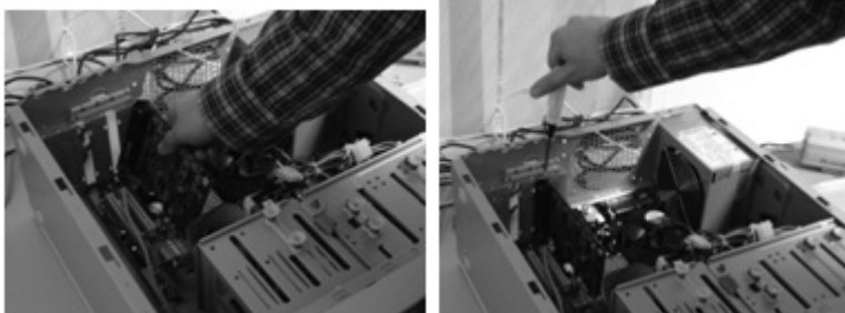
Example of FS-16 video capture card installation into a PCI-E X1 slot.
