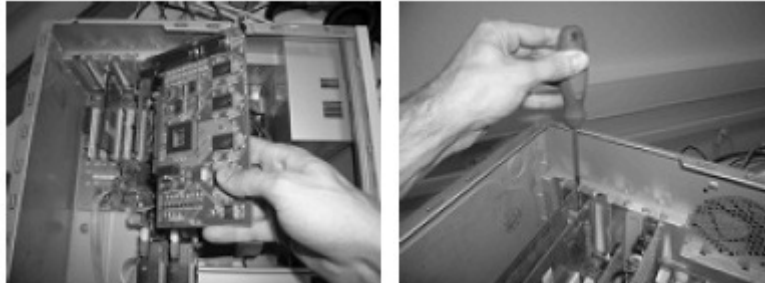
Example of FS-6C video capture card installation into a PCI slot.
