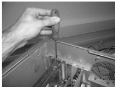
Example of FS-6C video capture card installation into a PCI slot.
