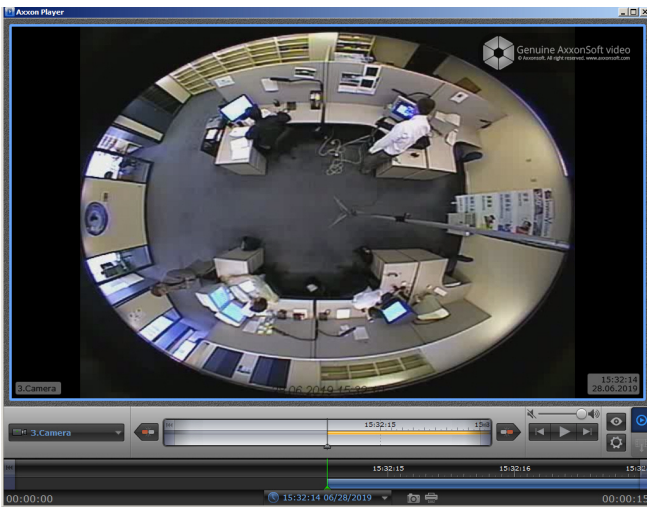
Video with the following conversion parameters: Lens: Standard fisheye lens, Position: Ceiling, Display: Perimeter:
