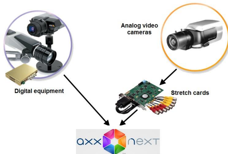
Fig. 1—1 A hybrid security system based on the Axxon Next software package
