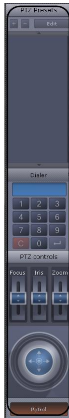
Fig. 6—5 The PTZ control panel
