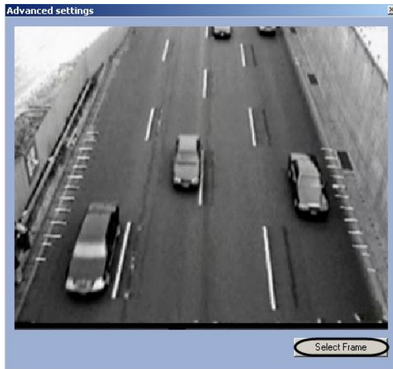
Fig. 7.4—5 Selecting the frame for markings setup
