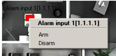
Fig.4.4-1 Alarm Input object's menu
