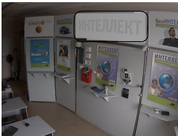
Fig. 6.5—4 A detection mask
