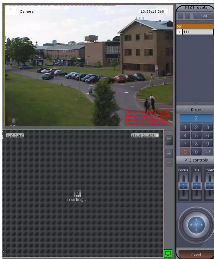
Fig. 7.3—27 The PTZ control panel
