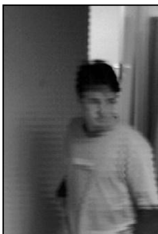
Fig. 7.3—11 An example of a combing distortion
