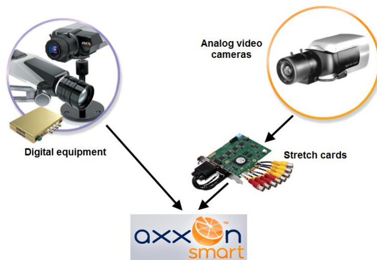
Fig. 1.3—1 A hybrid security system based on the Axxon Smart software package
