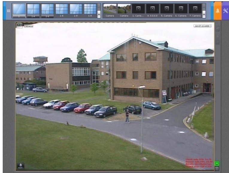
Fig. 7.3—1 Monitor with one viewing tile
