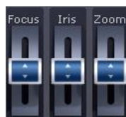
Fig. 7.3—33 The regulator scales for focus, iris, and optical zoom
