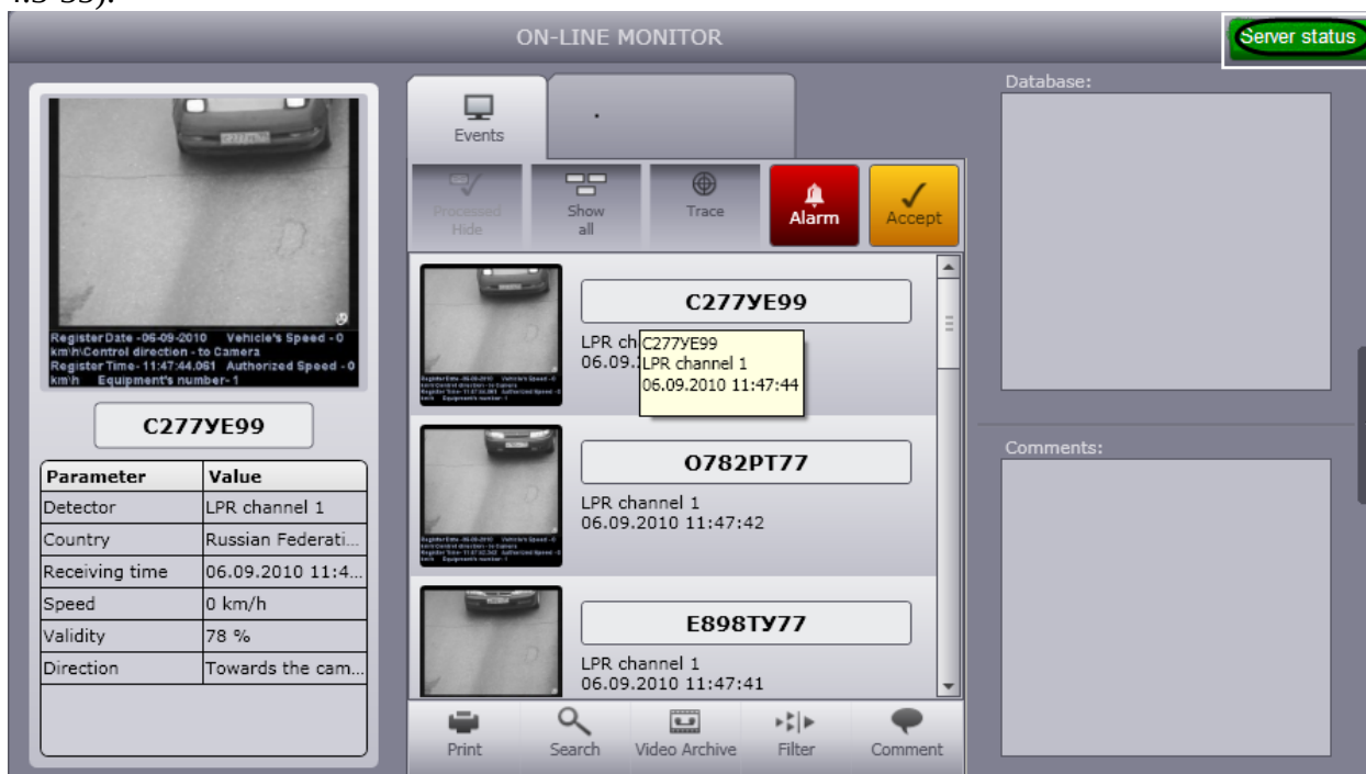
Fig. 4.3-33 Viewing the LPR channel errors
