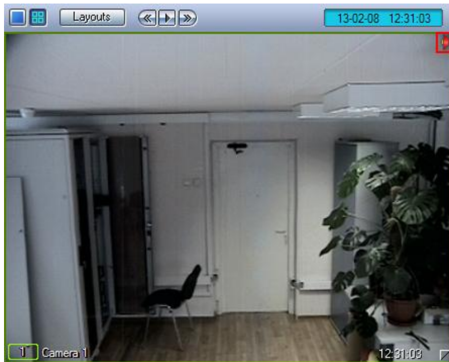
Fig. 4.4-2 Indicator of audio signal eavesdropping with the microphone (switched off) for synchro recordings
