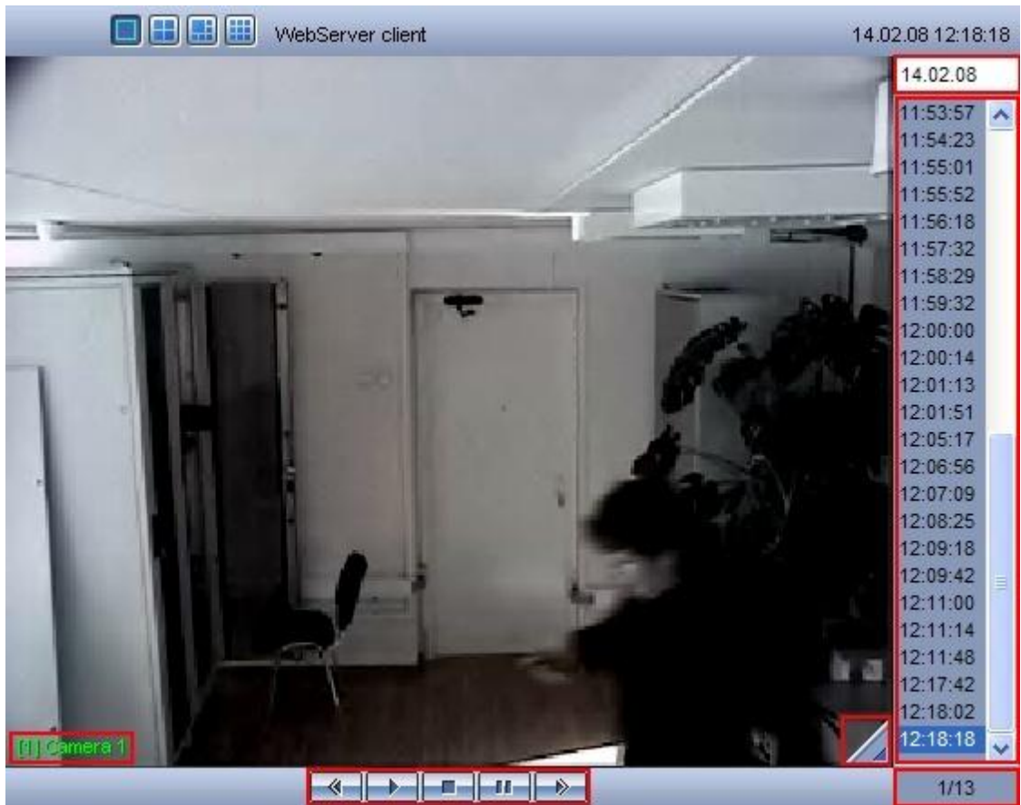
Fig. 4.16-10 Archive playback control panel interface for the Web browser
