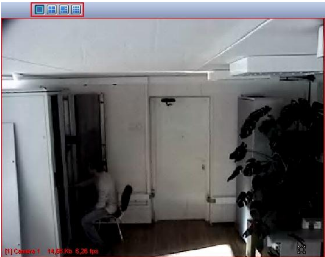
Fig. 4.16-4 Changing the number of surveillance windows within one Web browser monitor
