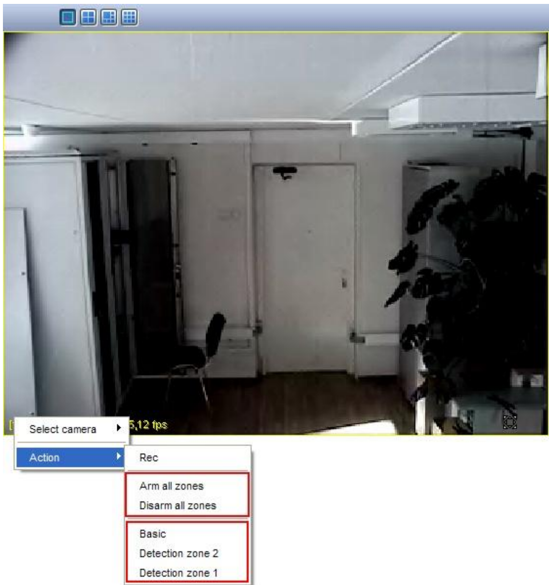
Fig. 4.16-7 Switching detectors on and off
