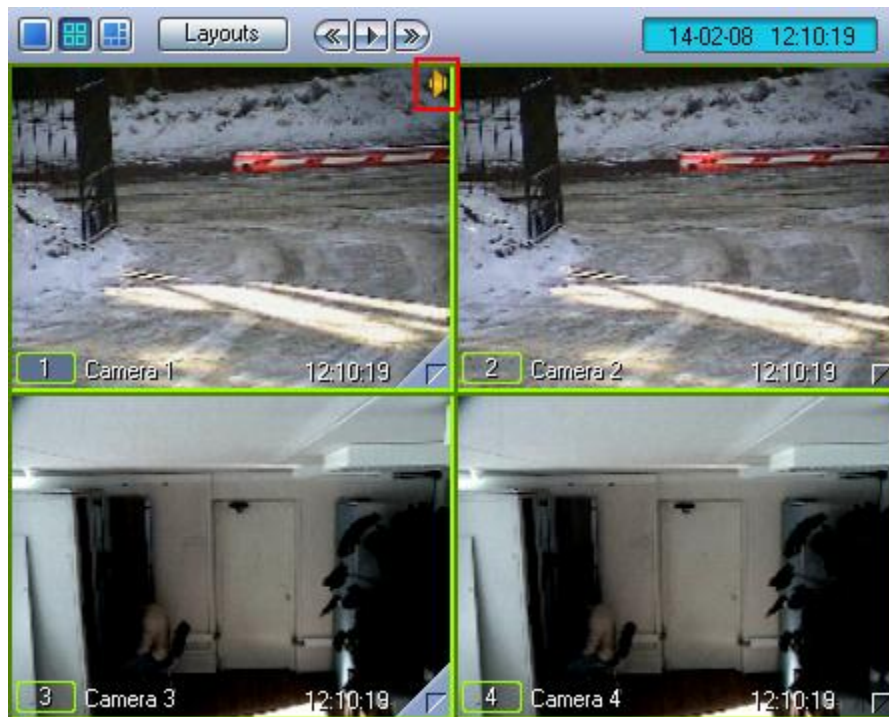
Fig. 4.3-26 The synchro audio recording and monitoring indicator
