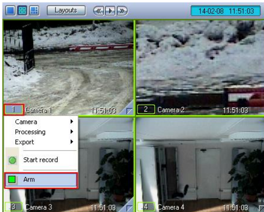
Fig. 4.3-8 Arming the camera by the main detector zone
