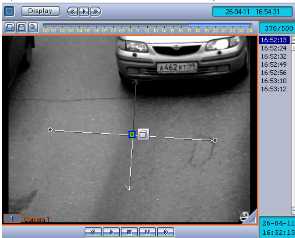
Fig. 4.3-57 Setting the traffic direction
