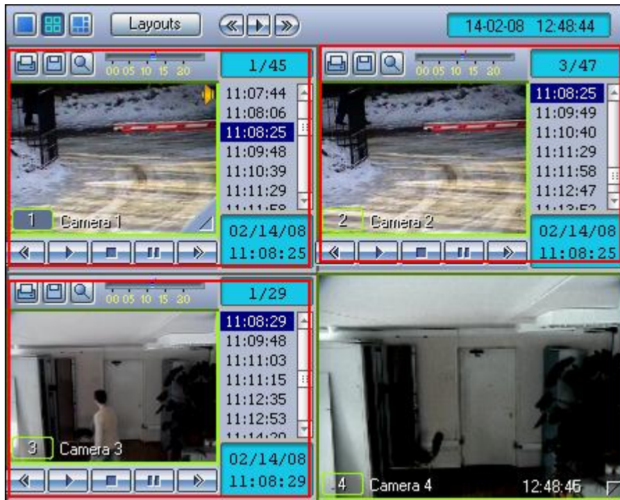
Fig. 4.3-70 Access to the synchro playback of a few video recordings
