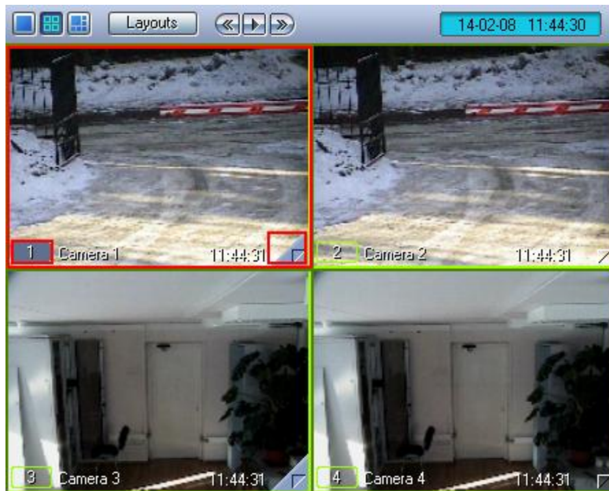
Fig. 4.3-4 Activated and de-activated surveillance windows
