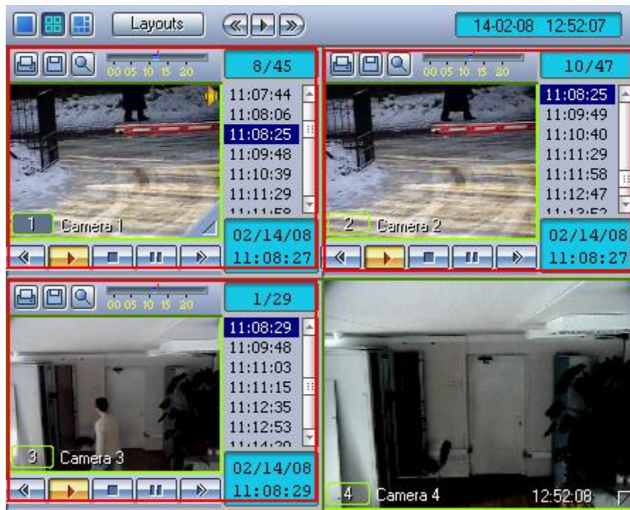
Fig. 4.3-72 Synchro playback of video recordings (playback is on)
