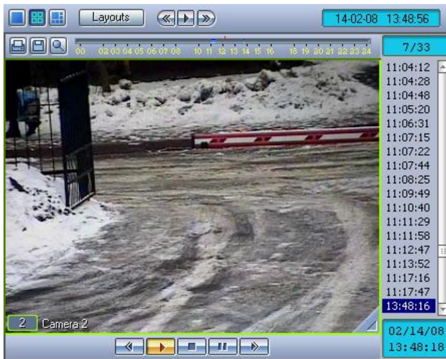
Fig. 4.3-60 The absence of indication of synchro audio recordings in the archive viewing mode.
