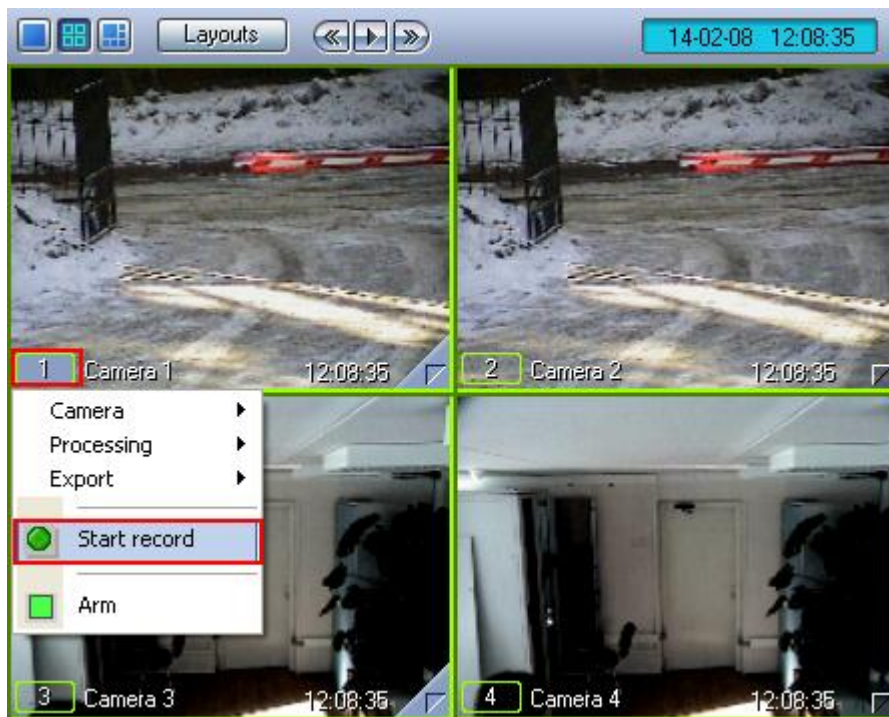
Fig. 4.3-24 Recording indicator in the video surveillance window functions menu (recording is OFF)
