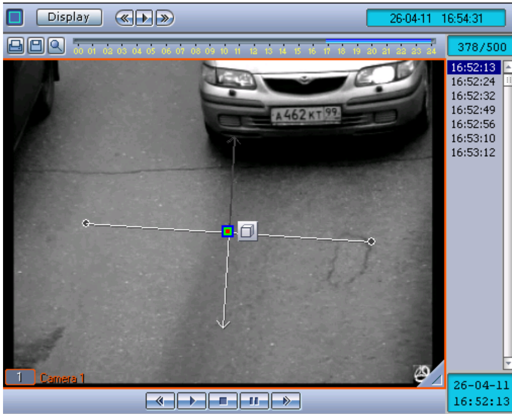
Fig. 4.3-60 Setting the traffic direction
