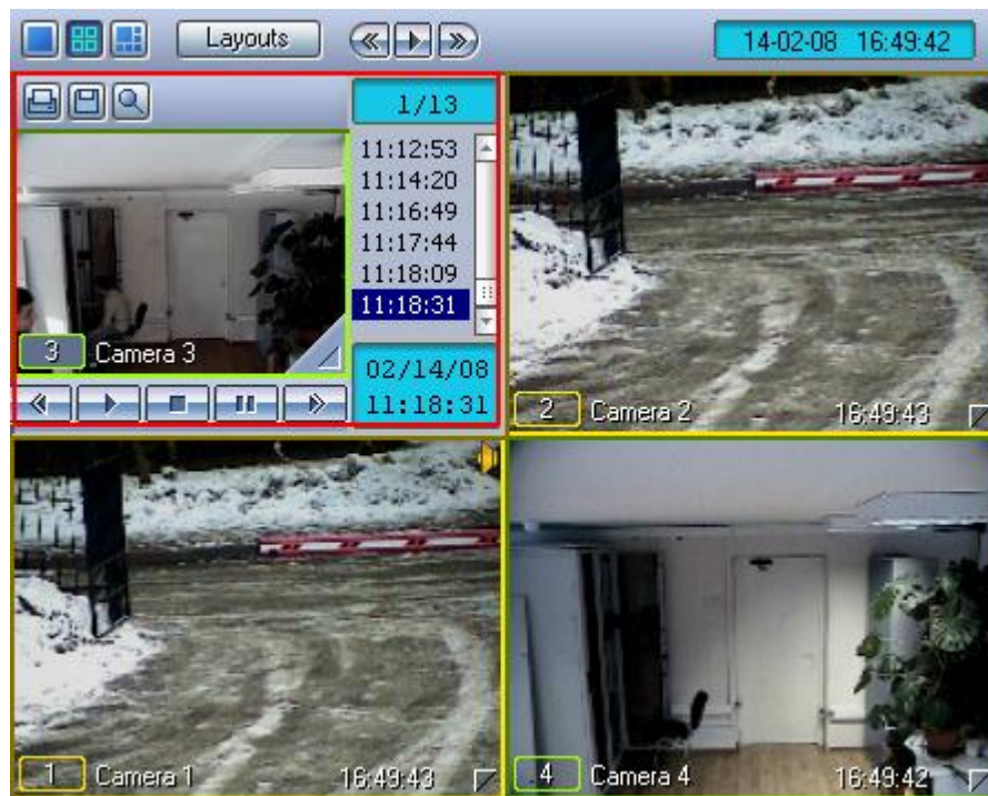
Fig. 4.3-46 Playback control panel of the backup archive generated by the active archive functional module
