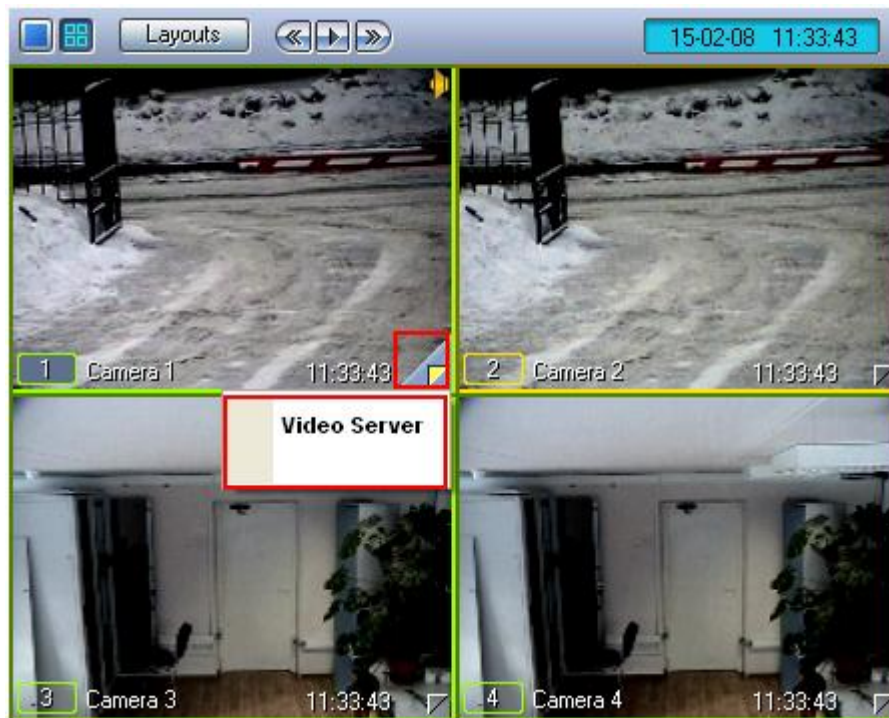
Fig. 4.3-52 Path to the main archive playback (where video gateway archive is available)
