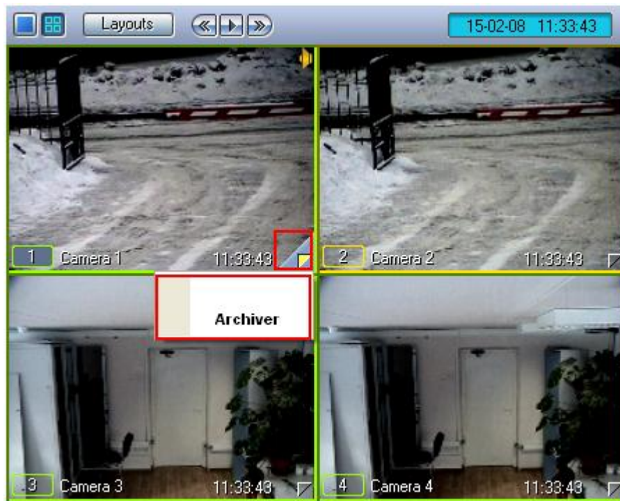
Fig. 4.3-45 Path to the playback of the main and backup archives generated by the active archive functional module
