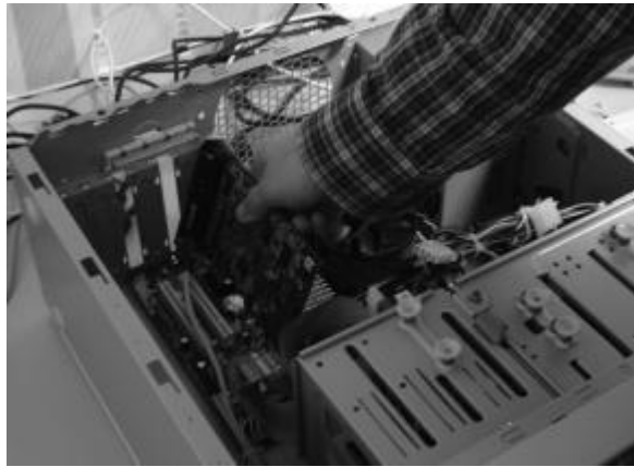
Fig. 2-1 Installation of video capture cards
