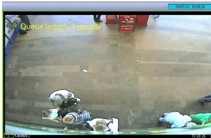
Fig. 7.1—1 Visualization of operating the Queue length detector
