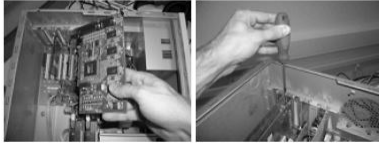
Figure 2.1-2 Example of FS-6C video capture card installation into a PCI slot
