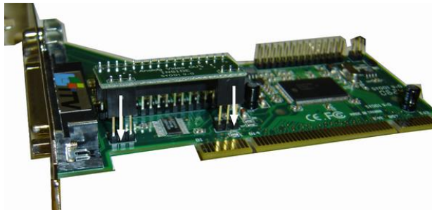
Figure 2.2-3 Connecting the analog video out card to corresponding connectors on the video capture card
