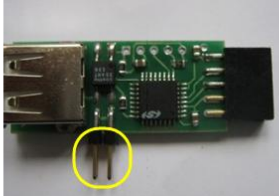
Figure 2.3-7 Appearance of the USB Watchdog hardware performance tester
