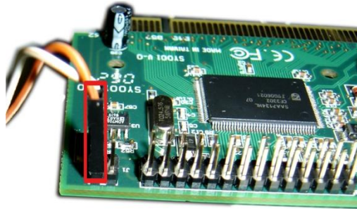
Figure 2.3-5 The Reset button cable connection to the four-pin connector of FS-5 video capture card
