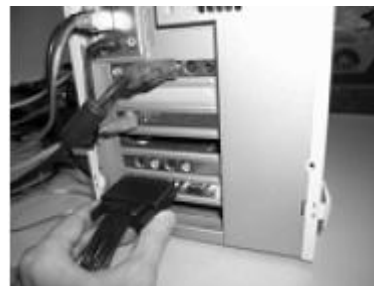
Figure 2.1-5 Connection of the interface cable
