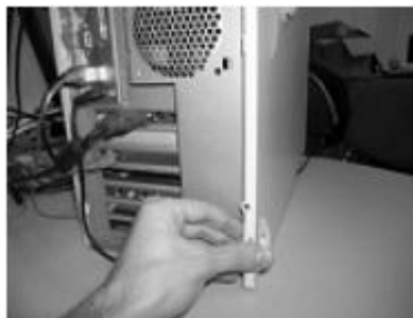
Figure 2.1-1 Removal of the case cover
