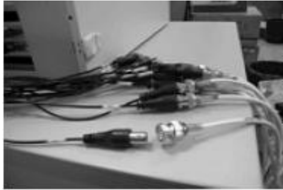
Fig. 2-3 Connecting video cameras to the BNC connectors
