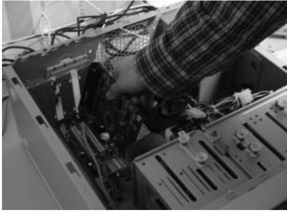
Fig. 2-1 Installation of video capture cards
